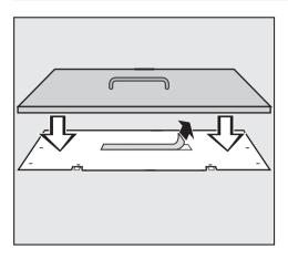
**6** Press the custom panel tightly onto the removed panel.
